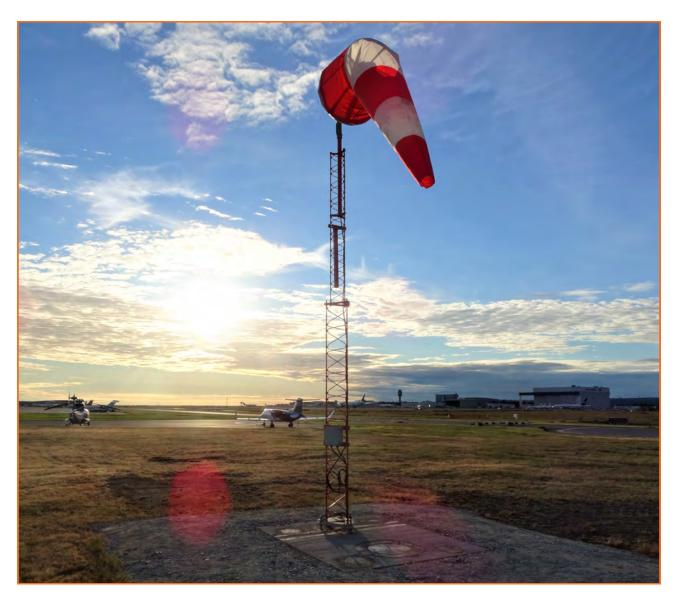
Millard Towers frangible Windsock towers rigidly support the heavy wind loading of windsocks, yet yield if accidentally impacted. Frangibility has been confirmed by third-party full-scale impact testing and FEA modelling. In fact, Millard masts are present in ICAO Doc 9157 as examples of proper frangible design and testing.
